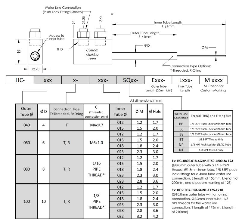
\*For SQBX option, the outer tube thread is BSPT For SQNX option, the outer tube thread is NPT
