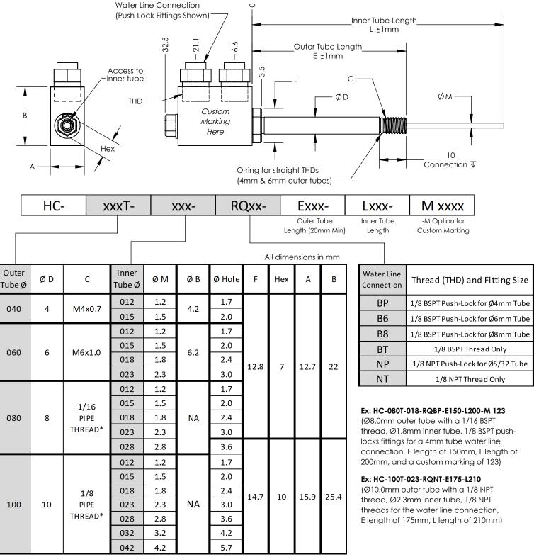
\*For RQBX option, the outer tube pipe thread is BSPT For RQNX option, the outer tube pipe thread is NPT
