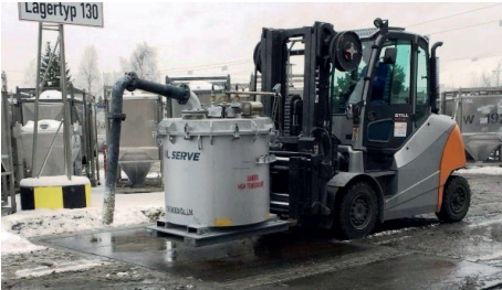
Liquid metal transfer with a sealed ladle offers an important safety during transits (no splashes) and drastically brings down the oxide and dross formation.
