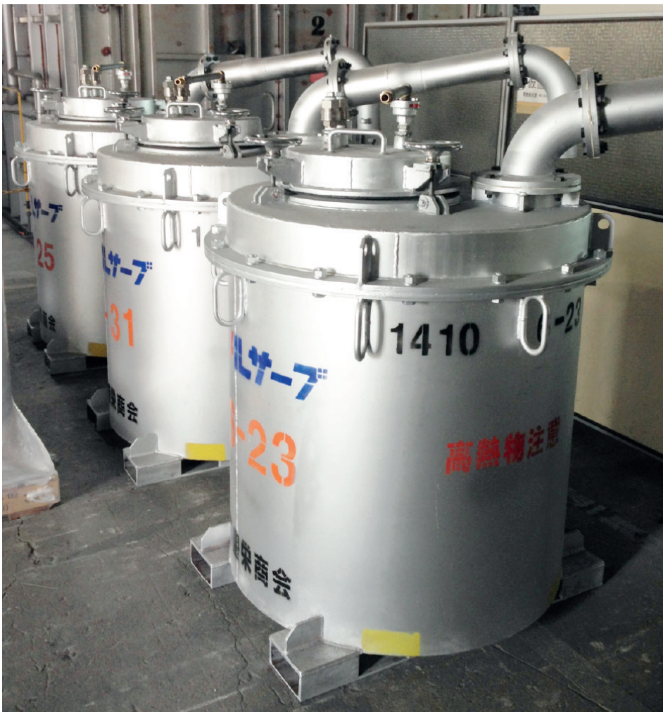
Filling of transfer ladle generates an average of 5.2 kg/Ton of oxides with standard pouring system, down to 0.9 kg/Ton with Al Serve vacuuming system.
