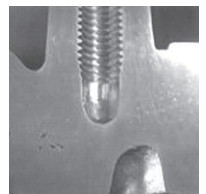
Casting when using jet cooling technology: decreased porosity
