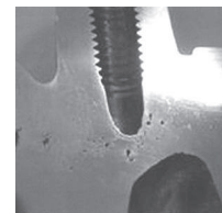
Casting without use of jet cooling technology : porosity occurs near thread
